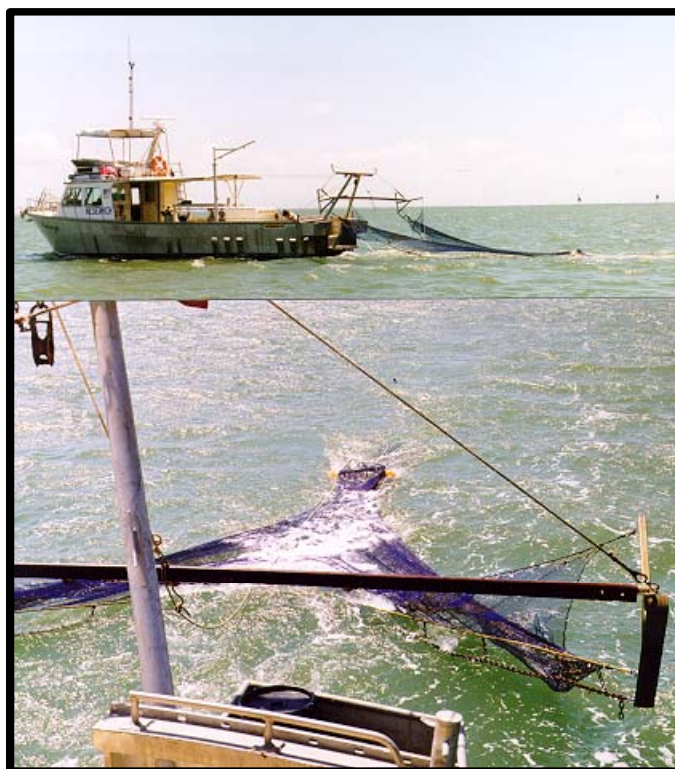
Figure 5.2.2 The QDPI RV Warrego and 5 m beam trawl used to examine fine-scale temporal and spatial effects on prawn catch rates.
